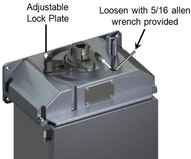
Figure 6 - Re-Position Locking Plate Manually
