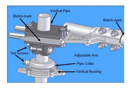
**Figure 8: Typical Operating Arrangement**
