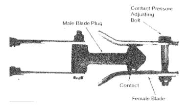
Figure 5: Contacts Shown Fully Closed
