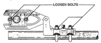
Figure 10: Top View of Adjustable Arm Assembly
