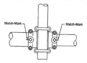
Figure 11: Match-Marked Hinge Clamp and Pipe
