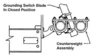
Figure 9: Counterweight Assembled
