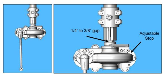
Figure 13: Type HOGO (High Output Geared Operator) Front View
