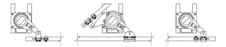
a. With the interphase pipe centered and all clevises in place, pierce the interphase pipe at the locations shown. Do not remove plastic caps at this time.
