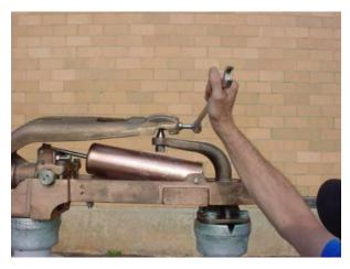
Figure 4: Switch Adjustment in Open Position
