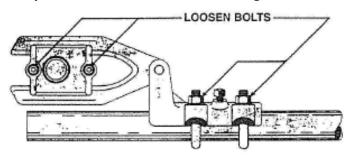
Figure 11: Top View of Adjustable Arm Assembly
