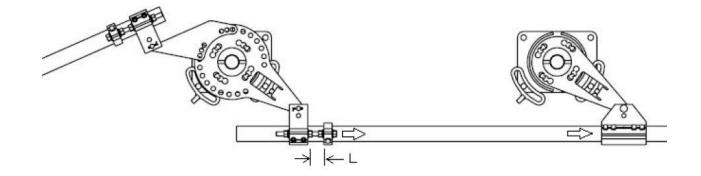
c. Set the timing of the last phase by adjusting the length "L" of the Rapid-Set clevis attached to the last phase.
