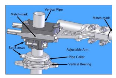
Figure 10: Typical Operating Arrangement
