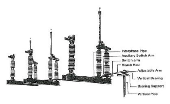
**Figure 8: Alternative Operating Mechanisms**
