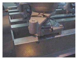
Figure 6: Bearing Stops
