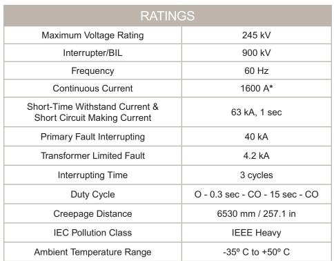
\*For applications above +40°C, continuous current rating shall be 1200A
