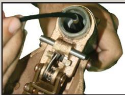
STEP 2: Insert tip of re-fusing tool into lower end of fuse tube. Push link through tube until ejector spring seats on counterbored shoulder inside fuse tube.
