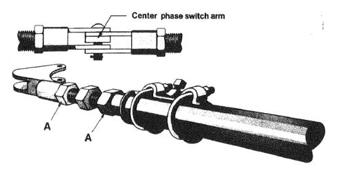
Operating mechanism adjustments consist mainly of incremental lengthenings and/or shortenings of the pipe that connect the switch arms together. To make these adjustments, simply loosen both jam nuts "A" and screw the stud in or out as required. Be sure to retighten both jam nuts securely.
