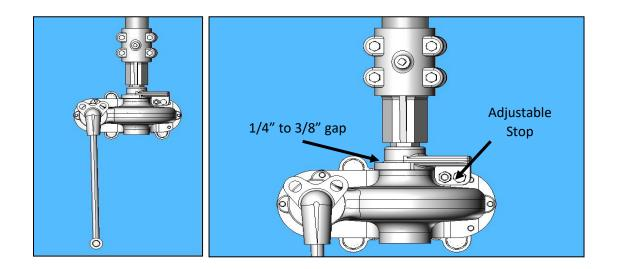
Figure 13: Type HOGO (High Output Geared Operator) Front View
