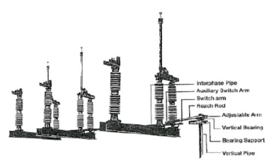
Figure 8: Alternative Operating Mechanisms
