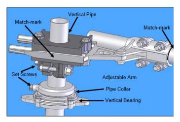
Figure 10: Typical Operating Arrangement
