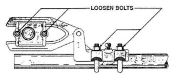
Figure 11: Top View of Adjustable Arm Assembly
