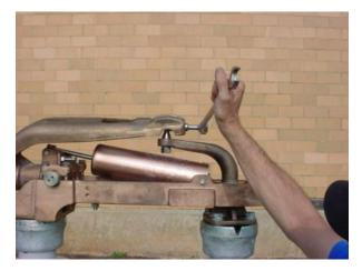
Figure 4: Switch Adjustment in Open Position
