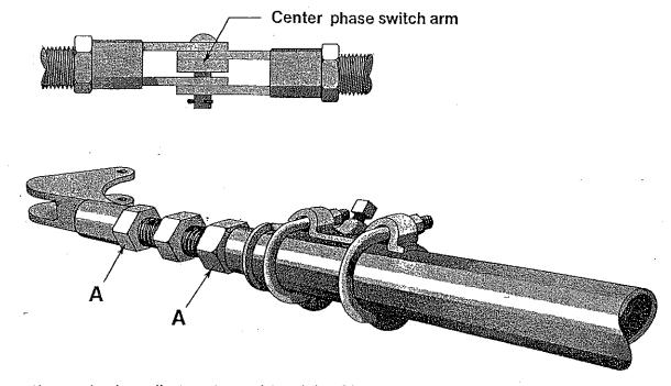
Operating mechanism adjustments consist mainly of incremental lengthenings and/or shortenings of the pipes that connect the switch arms together. To make these adjustments, simply loosen both jam nuts "A" and screw the stud in or out as required. Be sure to retighten both jam nuts securely.
