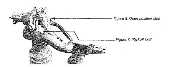
8. The "kickoff bolt" is an operating setting made and pinned at the factory. It should not be tampered with.
