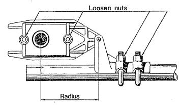
Figure 11: Changing the radius of the adjustable arm
