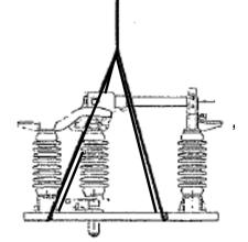
Figure 2<sup>-</sup> Recommended sling attachment
