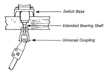
Figure 12: Vertical pipe attachment to the universal coupling
