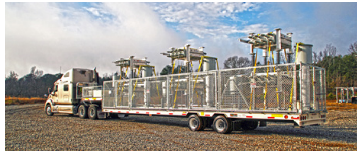
Mobile Capacitor Bank Trailer
