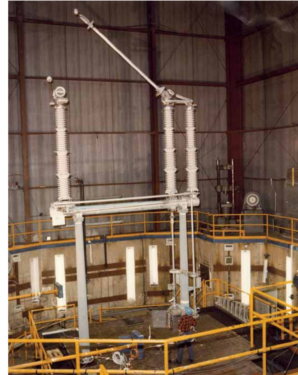
362 kV EV Disconnect Seismic Shaker Table Test, Wyle Laboratory, Huntsville, Alabama.
