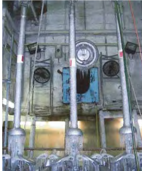
EV-2 242 kV 4000A Ice test – Switch Open (after icing).
