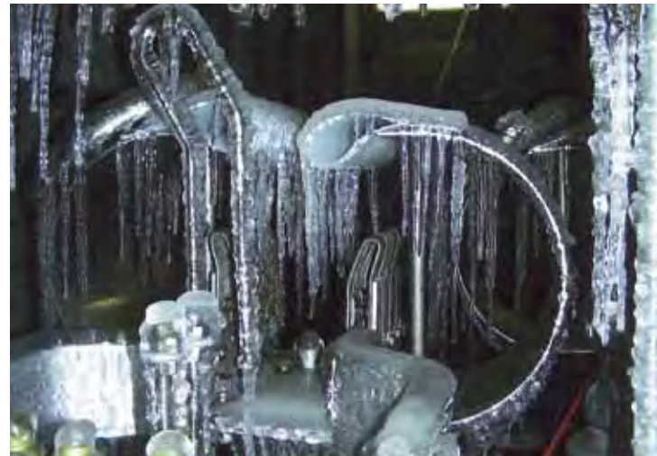
EV-2 242 kV 4000A Ice test – Switch Open (after icing).
