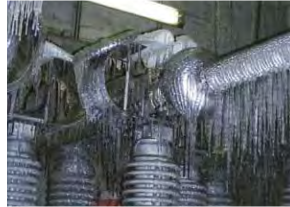
EV-2 242 kV 4000A Ice test – Switch closed (after icing).
