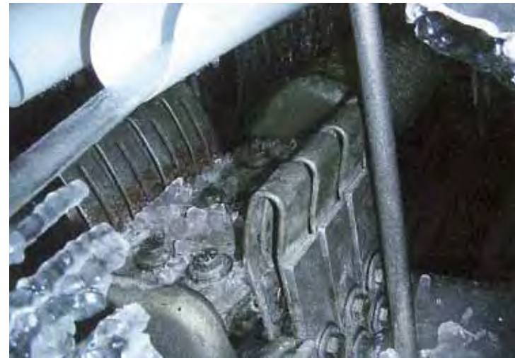
EV-2 242 kV 4000A Ice test – Switch after closing operation.
