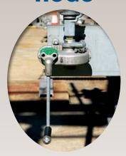
The newly redesigned HOGO provides an anti-back drive feature which prevents operator injury caused by "free wheeling." Its round shaft allows for roller bearings which reduce slop, includes loading capability, and improves sealing.
