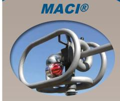
Southern States' **MACI®** is a magnetically actuated closed indicator that verifies the blade of a disconnect switch is correctly placed in the jaw and properly rotated. This binary indication helps operators ensure that the switch is safe to energize.
