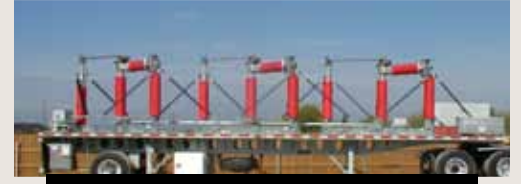
145kV CSH-B fixed to a modified flat-bed trailer
