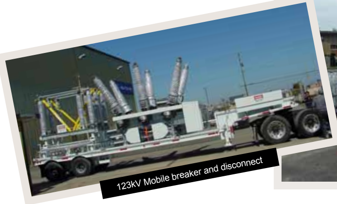
CSH-B all composite interrupters, support insulators and lightning arrestors
