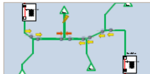
Control Center SCADA Display with Fault Direction Indication
