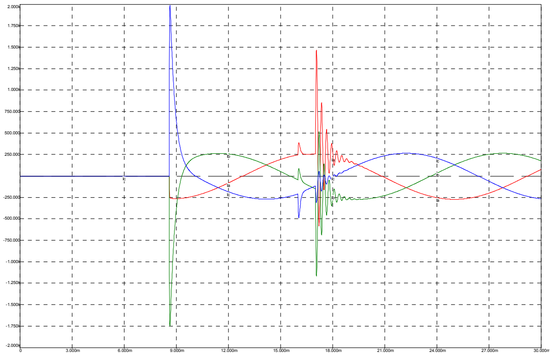
Capacitor Currents from Simulation for U. S. Utility Installation of Capacitor Switch using Pre-Insertion Resistor
