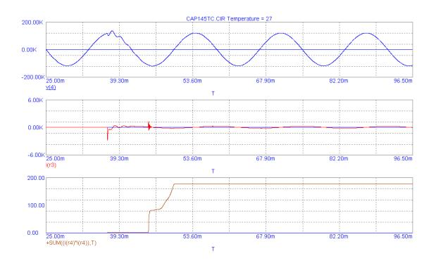
Proposed Configuration (With Overvoltage Control) With *CapSwitcher*<sup>®</sup> Having 40 Ohm Pre-Insertion Resistor Being Used On The First Bank Switched – First Bank Switching <u>Without</u> Inductors (Simulation 4) - First Bank Energized = 104 ( $I^2t$ ) Main Contact Arcing Energy
