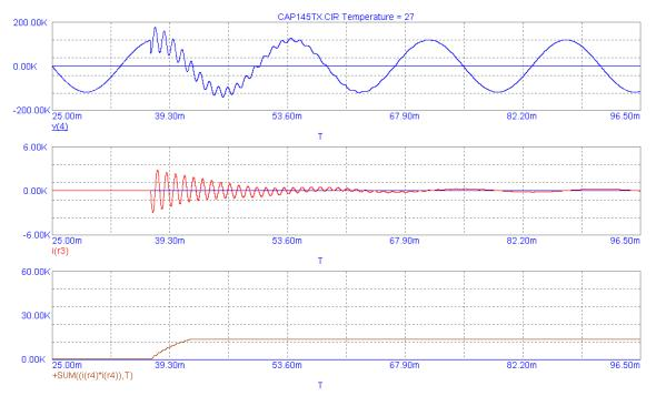
Example Standard Configuration – First Bank Switching with Inductors (Simulation 2) – First Bank Energized = 13,554 ( $I^2t$ ) Main Contact Arcing Energy
