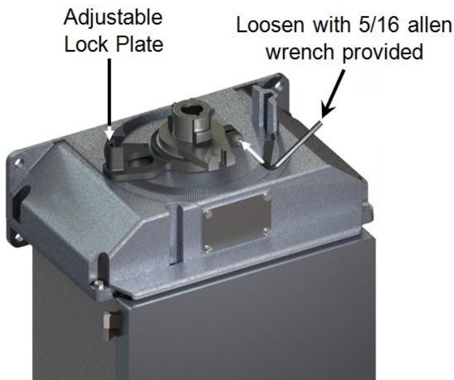
Figure 5 - Re-Position Locking Plate Manually
